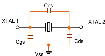
$$CL = C_g \times C_d / (C_g + C_d) + C_s \text{ (pF)}$$
