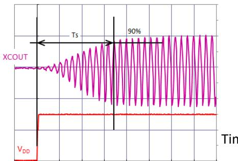
Time from the application of VDD until the XCOUT amplitude reaches 90%
